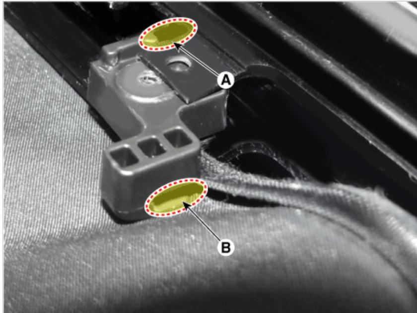
9. Loosen the roller blind shoe clip mounting screw (A).
