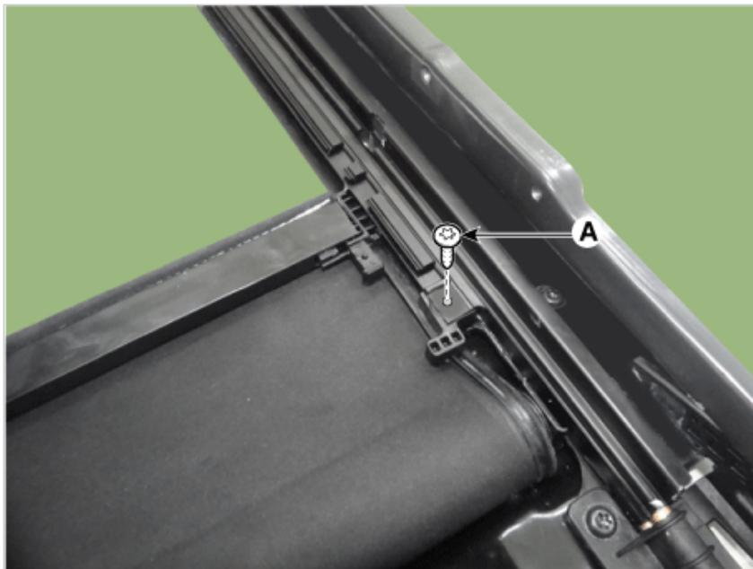
8. Remove the roller blind lead (A) from the mechanism rail.
