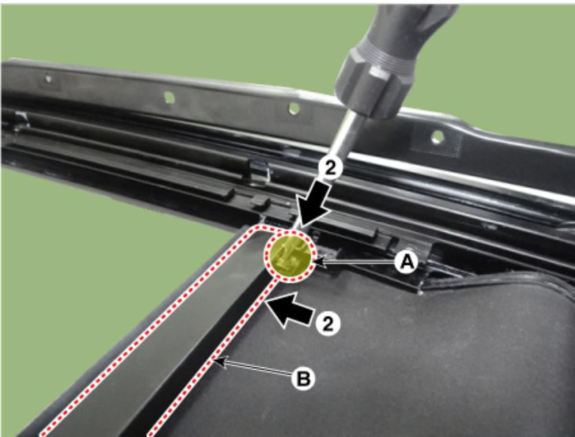
12. Separate right side of the roller blind (A) by pushing washer (B).
