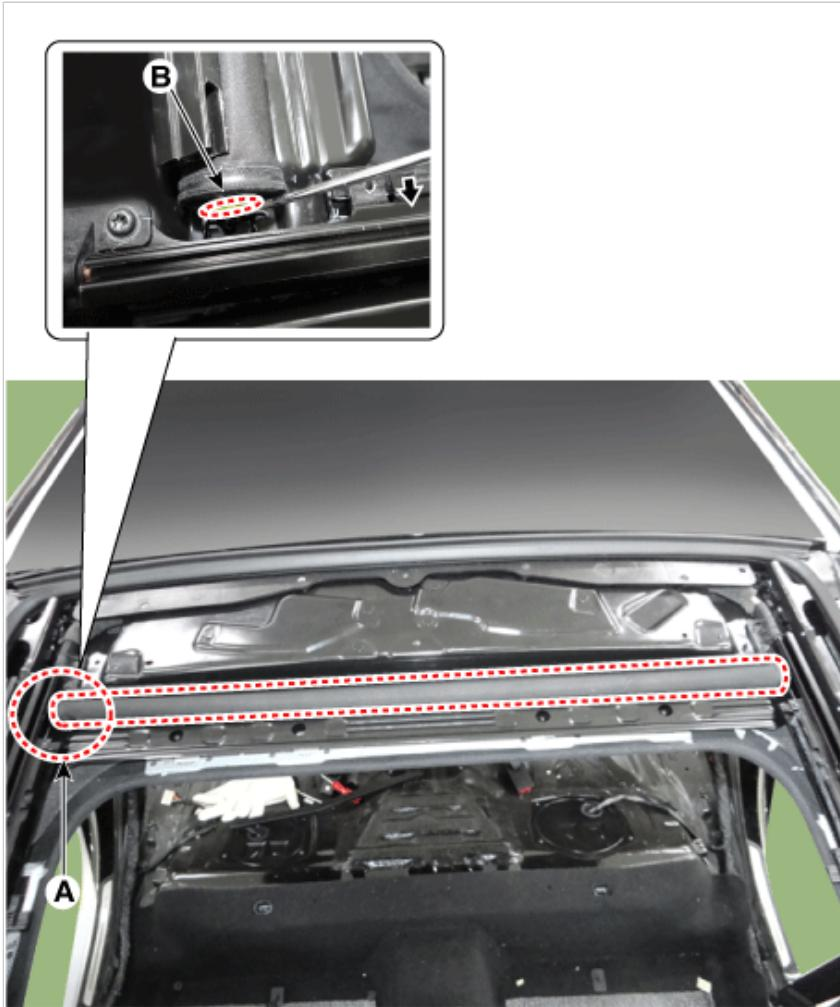
13. Remove the roller blind (A) after separating the roller shaft (B) from the sunroof assembly.
