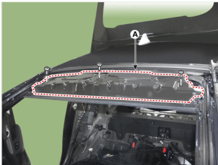
7. Loosen the roller blind lead mounting screw (A).
